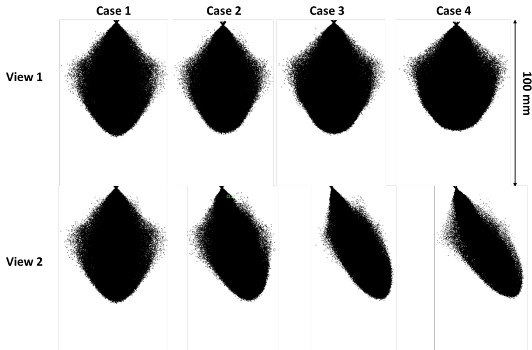
Figure 8.14: Spray structure for four different cases in both View 1 and View 2.
