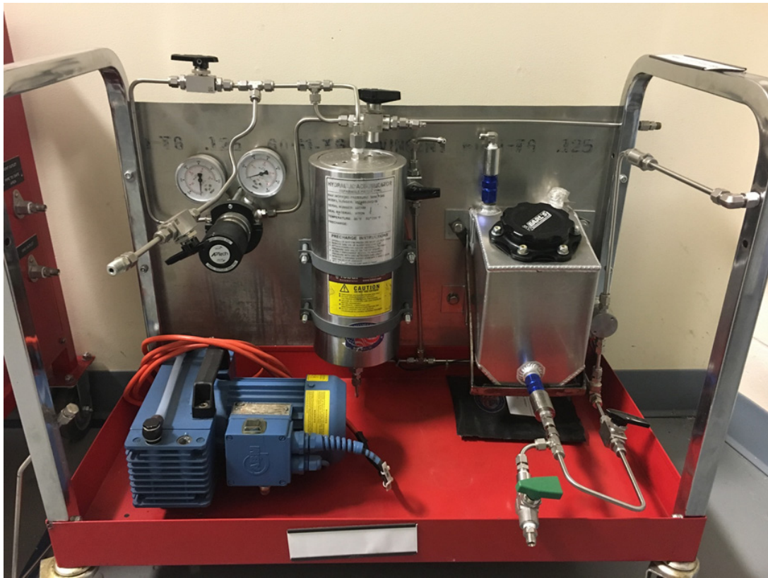
Figure 3.2: Low pressure fuel delivery system.
